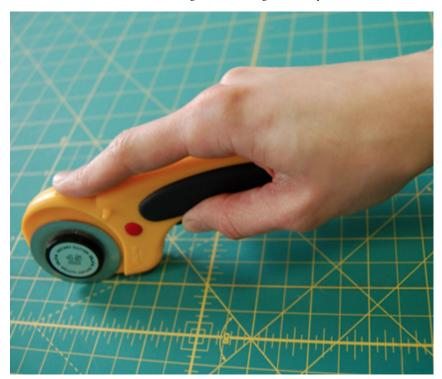
Here is the cutter and my hand in cutting position. The safety is off and I am squeezing the black lever, which pushes out the blade. My hand and wrist make a nice straight line and my index finger is pressing against the non-slip section on the top. Some people prefer to keep their index finger on the right side of the cutter or against the black lever, but whichever way you prefer it's important to keep your wrist straight. This will help prevent a repetitive motion injury.
